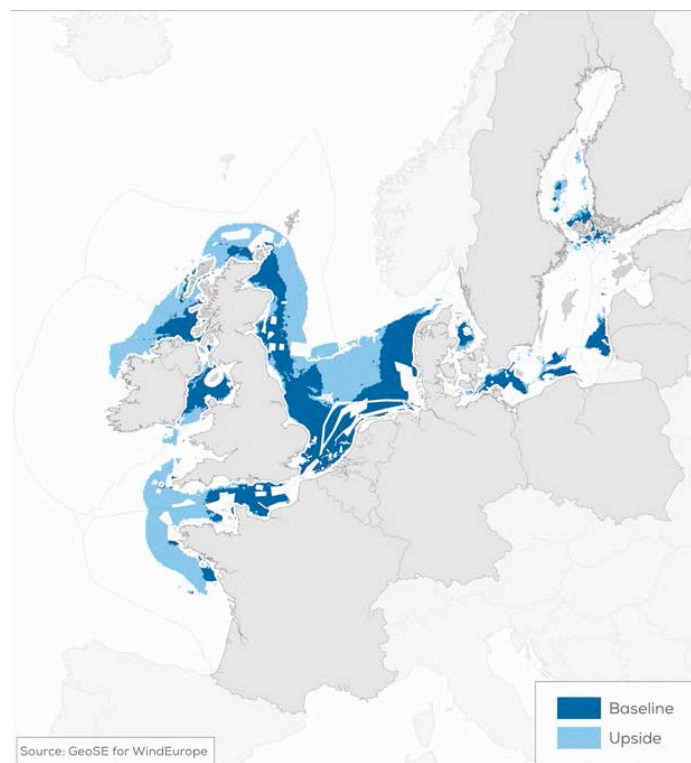
Figure 2: Wind farm areas defining an economic potential up to € 65/MWh under the baseline and upside scenarios
